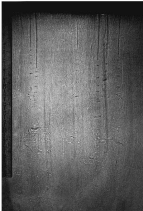
FIGURE 3. Photographs taken during an experiment in which an aqueous solution of sodium chloride (3.55 wt%) was cooled and solidified from above at a base-plate temperature of T_B = -15^\circ\text{C} . A centimetre scale is shown on the left. The black region at the top of the photographs in (a), (b), and (d) is the mushy layer. (a) Early in the experiment, when the mushy layer has a depth of 2.4 cm, weak interfacially driven compositional convection is evident in the form of very thin streamers. These emanate mainly from the interfacial region between the mushy layer and the liquid and do not carry a significant flux of salt (see figure 6). (b) Later in the experiment, when the depth of the mushy layer is about 11.5 cm, which is greater than the critical
