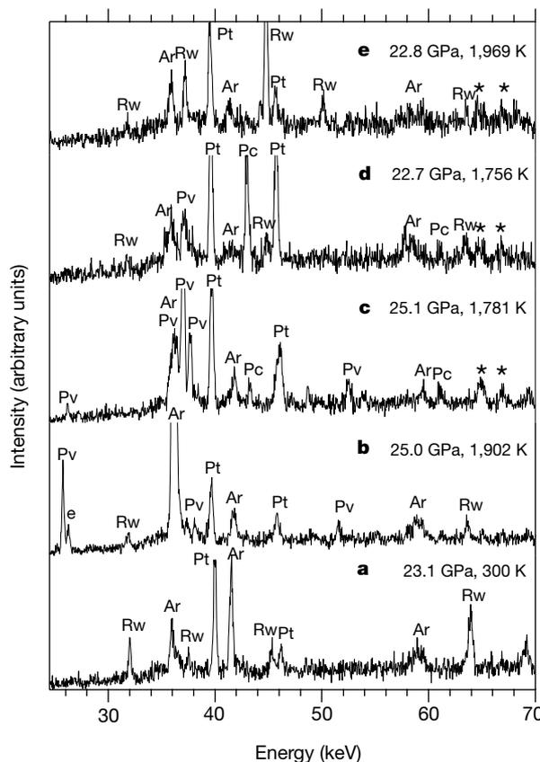
Figure 1 a–e, Representative X-ray diffraction patterns at the indicated *P–T* conditions. Peak identifications are: Rw, ringwoodite; Pv, perovskite; Pc, periclase; Pt, platinum; Ar, argon; asterisk, platinum fluorescence; e, detector escape peak.
