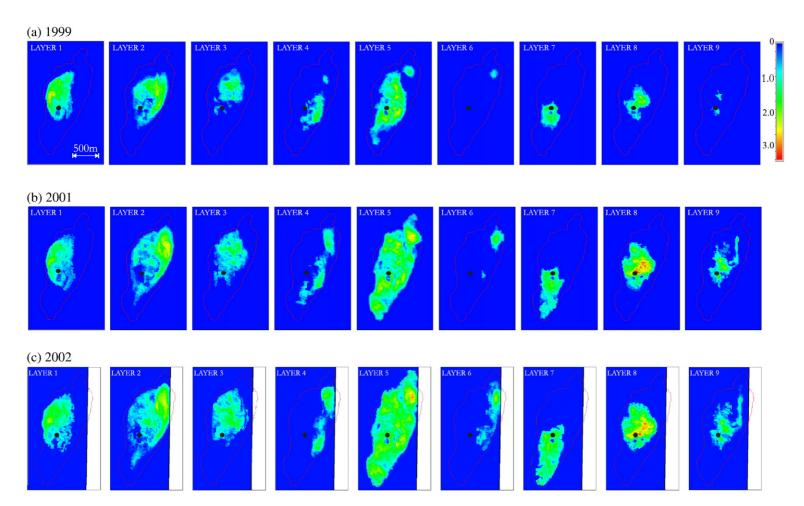
Fig. 4. Maps showing the relative seismic amplitude of the bright reflections on the 1999, 2001 and 2002 seismic surveys. These correspond to the tops of the CO<sub>2</sub>-saturated layers. Black spot corresponds to injection point. Red polygon denotes full areal extent of 2002 plume.
