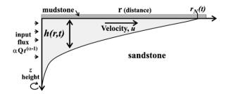
Fig. 3. Model for gravity driven flow of a less dense viscous fluid introduced along axis at r=0 into a porous medium initially filled with fluid of higher density. Note that only the density differences and the horizontal motions are taken into account and that viscous flow in the fluid initially filling the sandstone is ignored.
