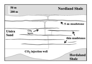
Fig. 1. Schematic illustration of  $\mathrm{CO}_2$  injection at Sleipner and rising  $\mathrm{CO}_2$  plumes being partially trapped under thin mudstones before reaching Nordland Shale cap rock. Note the vertical exaggeration.
