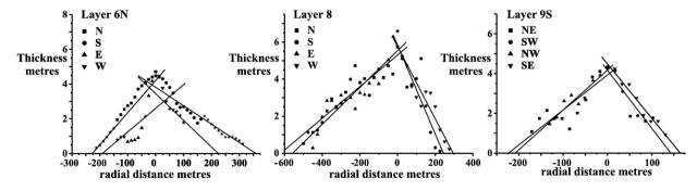
Fig. 7. Thickness of layers 6N, 8 and 9S calculated from 2002 seismic survey plotted against radius for two orthogonal profiles. Lines are least squares fits used to calculate the magnitude of the local radius of each CO<sub>2</sub> accumulation which are then used to normalise radial distances (see text). The stars in plot of layer 6N are points used in regression.
