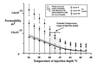
Fig. 10. Estimated permeabilities from whole-reservoir model and thickness-radius data from layers 6N, 8 and 9S as a function of temperature at injection depth.  $2\sigma$  error bars reflect only uncertainties in least-squares fits to radius and thickness-radius data (Figs. 4 and 8). Most probable temperature at injection depth is  $41\pm1$  °C.
