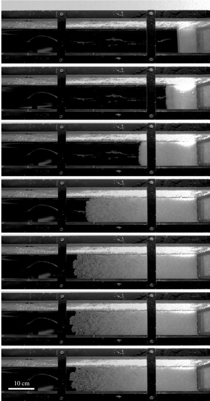
FIGURE 3. Top view of the spreading beads in a representative experiment. The propagating front remains almost uniform across the width of the tank until the current is close to its final length. The pictures were taken at t = \{0, 0.6, 1.8, 6.0, 10, 20, 30\} s. The experimental parameters are the same as the experiment in figure 2.
