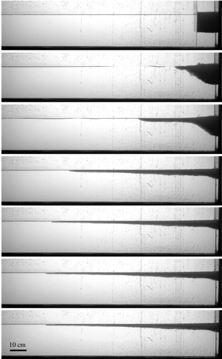
FIGURE 2. Side views of the spreading beads in a representative experiment (experiment 2a in table 3). The pictures were taken at t = \{0, 0.6, 1.8, 6.0, 10, 20, 30\} s. The tank was filled with saturated salt water of depth d = 15 \pm 0.1 cm, m = 765 \pm 1 g and x_i = 10 cm. The pictures show the initial spreading with time followed by the front coming to a halt.
