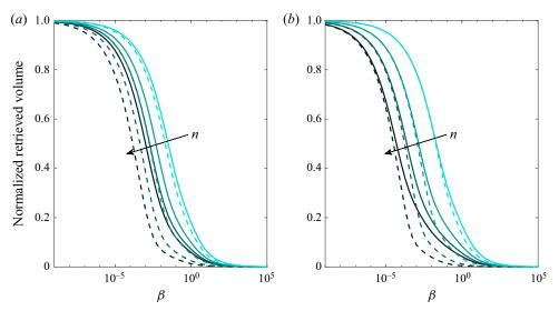
Figure 9. Comparison of drainage from either the left (solid curves) or right (dashed curves) ends of non-branching networks of various size (n = 2, 4, 6, 8), showing the relative fraction of initial fluid volume retrieved at varying non-dimensional permeability  $\beta = H^{*-3}$ . (a) Rigidity factor  $\eta = 1.1$  and uniform permeability, i.e.  $\kappa = 1$ . (b) Permeability factor  $\kappa = 2$  and uniform rigidity, i.e.  $\eta = 1$ .
