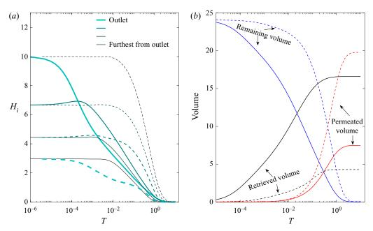
Figure 8. Results for a non-branching network with n = 4 generations, initial outlet aperture  $H^* = 10$ , and rigidity factor  $\eta = 1.5$ , comparing drainage from either the left softer (solid lines) or right more rigid (dashed lines) ends. (a) Evolution of the aperture. (b) Evolution of the volumes of fluid remaining in the network, retrieved via the outlet, and lost via permeation through the channel walls.
