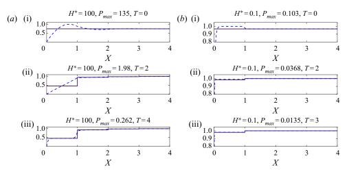
Figure 4. Non-dimensional numerical solutions of pressure  $P(X, T)/P_{max}$  (dashed lines) and aperture  $H(X)/P_{max}$  (solid lines) for a network (n = 4) with two different magnitudes of initial condition: (a)  $H^* = 100$ ; (b)  $H^* = 0.1$ . The results are scaled using the instantaneous maximum pressure  $P_{max}$ .
