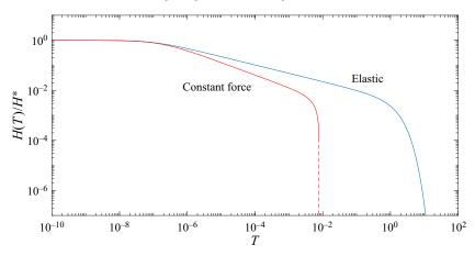
Figure 6. Comparison for a single channel between our model (with  $H^* = 100$ ) and a similar model with a constant force of non-dimensional value  $H^* = 100$ , so that at T = 0 the applied force in both models is the same. The dashed vertical line denotes the contact time, i.e. H(T) = 0, in the constant-force model.
