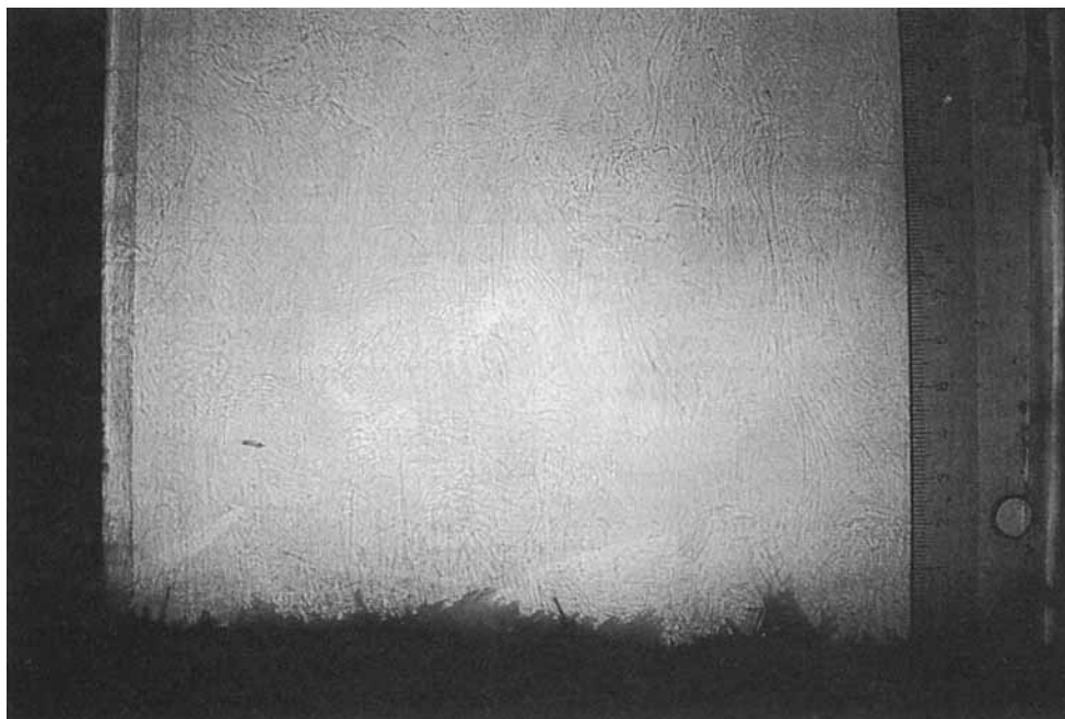
FIGURE 3. Shadowgraph of the compositionally driven convection during an experimental run.
