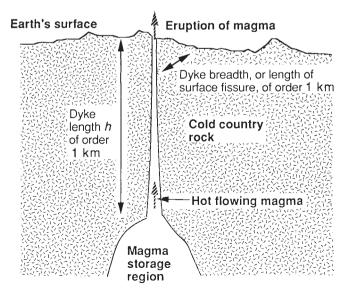
FIG. 1 Cross-section through a typical sheet-like planar dyke. Note that the dyke need not necessarily be vertical.
