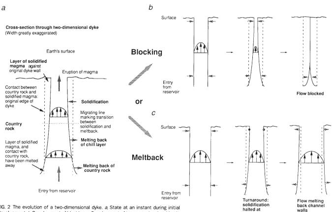
FIG. 2 The evolution of a two-dimensional dyke. a, State at an instant during initial development. b, Development of blocking. c, Development of turnaround and meltback.
