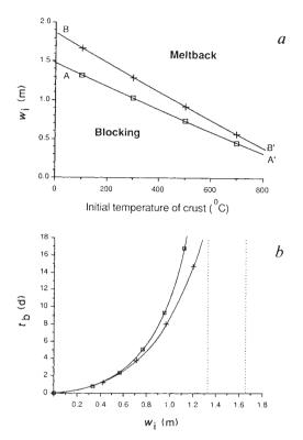
FIG. 3 Numerical results of model, for parameter values given in text. *a*, Regions of parameter space in which blocking or meltback are predicted for dyke length 2 km (squares) and 5 km (crosses). *b*, Time for dyke to become blocked as a function of initial dyke width, for  $T_{\infty} = 100$  °C. The time to block becomes infinite for widths approaching the critical value for meltback to occur (dotted lines (left) H = 2 km; dotted lines (right) H = 5 km). Symbols as in *a*.
