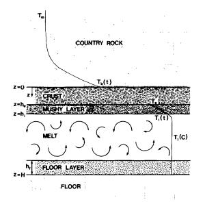
Fig. 1. Schematic diagram of an intrusion being cooled from above. Heat is conducted into the country rock above the roof at z = 0. As the magma is cooled it crystallizes to form a crust of composite solid above a mushy layer. The molten magma convects vigorously as it cools with internal crystallization producing a solid layer near the floor. A sketch of the temperature field is indicated on the diagram.
