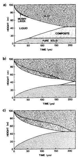
Fig. 5. The growth of solid as a function of time for magma in a chamber 100 m high intruded at its liquidus into country rock at 0 °C. The three diagrams indicate the different evolutions experienced by intrusions of different initial compositions  $C_0$  and hence liquidus temperatures  $T_L$ . (a)  $C_0 = 65\%$  Di,  $T_L = 1308$  °C; (b)  $C_0 = 80\%$  Di,  $T_L = 1352$  °C; (c)  $C_0 = 95\%$  Di,  $T_1 = 1382$  °C.
